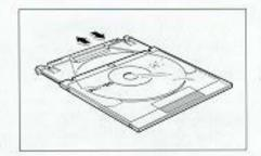
The reverse action removes the disc after use. The box is inserted into the slot, as before, and the disc and its frame are relocated within the box (inside the player) ready for withdrawl. The box is now slid outwards with the disc already contained inside. This caddy facility avoids physical handling of the media and provides a practical, robust and compact storage element.
